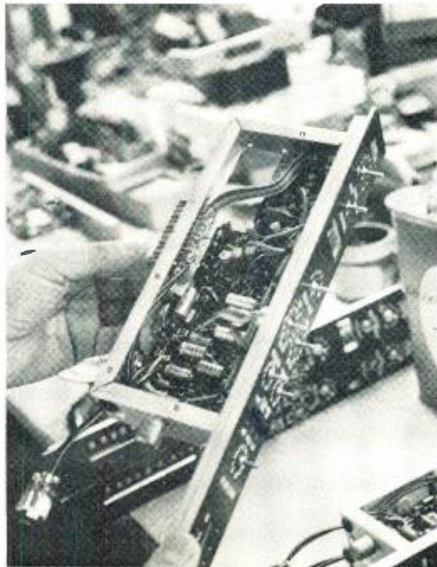
Fader module gets final look-over before cover plate goes on and unit goes onto the shelf.
